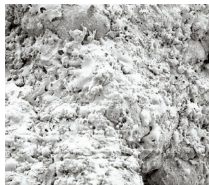
SEM pictures of a HA-sprayed surface
